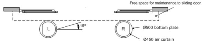
COMPACT400 has a fixed outblow angle of 15°. The special shaped bottom plate makes it possible to increase the angle up to 30°.
