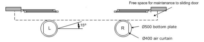
COMPACT400 has a fixed outblow angle of 15°. The special shaped bottom plate makes it possible to increase the angle up to 30°.
